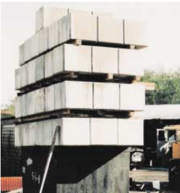
77,500# test load on top of a septic tank Septic tank vacuum test to 7" Hg (=500 psf force on all 6 sides)
