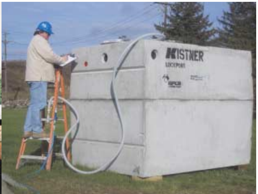
77,500# test load on top of a septic tank Septic tank vacuum test to 7" Hg (=500 psf force on all 6 sides)
