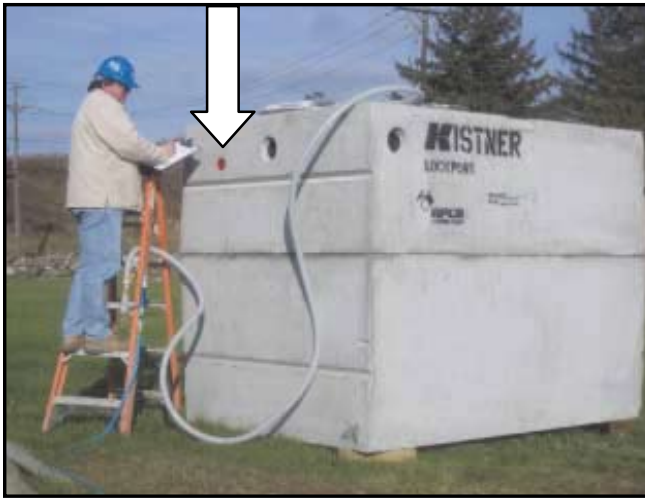
Vacuum testing a PCANY Certified Tank
