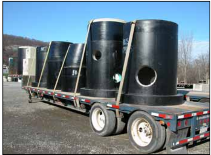
Precast manholes ready to ship
