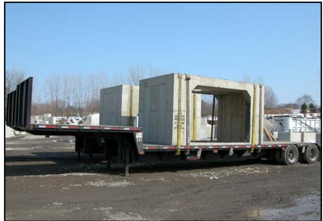
Meadowlands drainage structures, with diagonal corners to strengthen large openings
