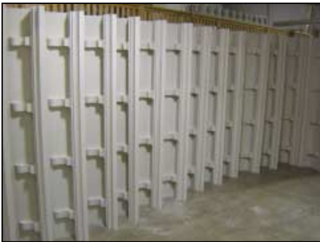
Finished cornice sections awaiting shipment
