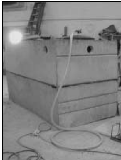
Septic tank undergoing plant vacuum test
